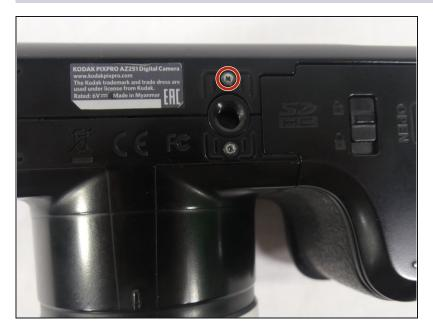
Remove the single 5mm Phillips #00 screw from the bottom.
