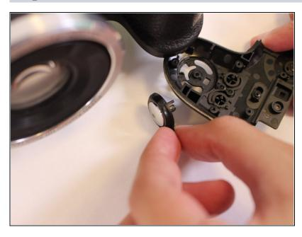
• Remove the shutter button by pulling it out from the bottom side of the top cover.
