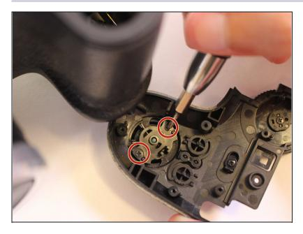
• While holding the shutter button in place, remove the two 4mm JIS #000 screws from the base.
