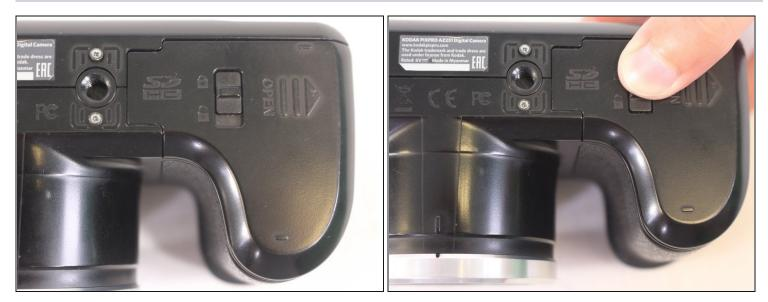
• Slide switch to open lock position.
