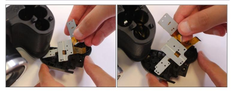
• Remove the metal base and ribbon cables.
