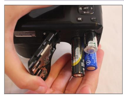
• Remove the batteries.
