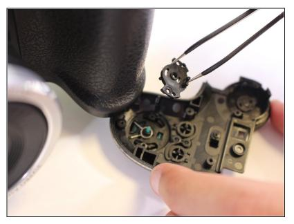
• Remove the plastic base of the shutter button using tweezers by pulling it straight upward.
