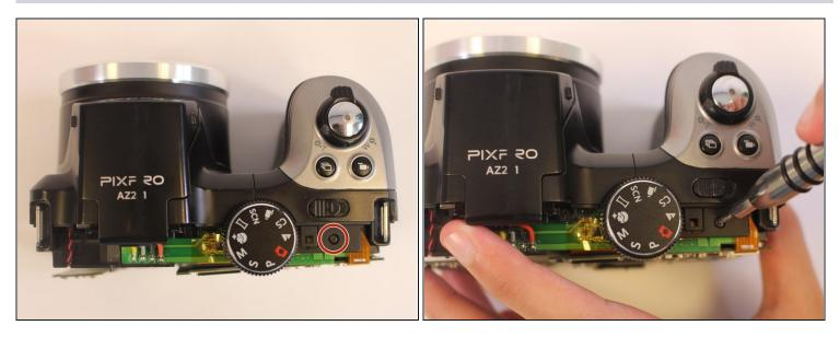
• Remove one 4mm JIS #000 screw from the top of the camera.
