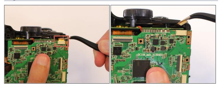
• Using <u>tweezers</u>, disconnect the orange cable connection at the top of the motherboard.
