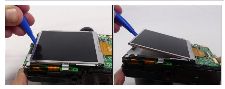
• Pry the LCD screen out of the metal housing plate with a plastic opening tool.
