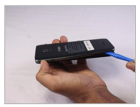
Using a plastic opening tool, pry the back cover off of the phone.
