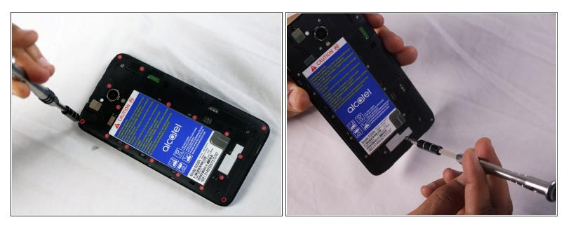
Remove the seventeen Phillips #000 screws from the mid-frame.
