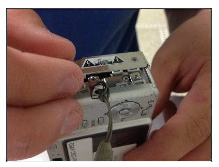
• Lift the side panel of the camera up to release the front case.
