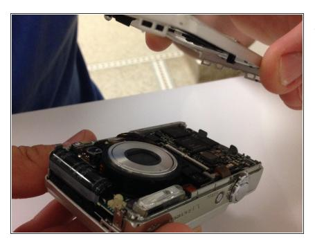
• Lift the front case up gently to remove it completely.
