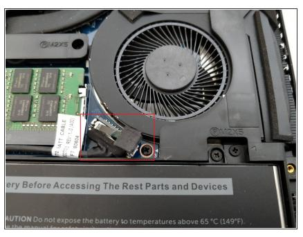
To disconnect the battery, pull gently upwards on the tab connector.
