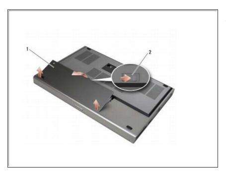
Slide the battery release latch and remove the battery.
