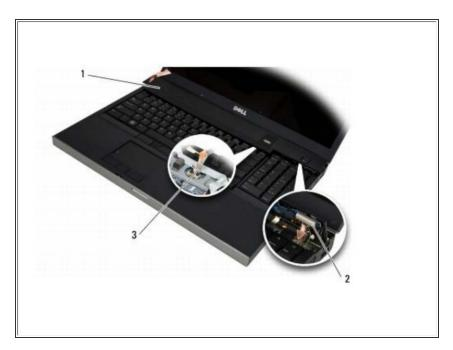
Starting on the left, gently lift the LED cover and disconnect the power cable and the biometer cable if present.
