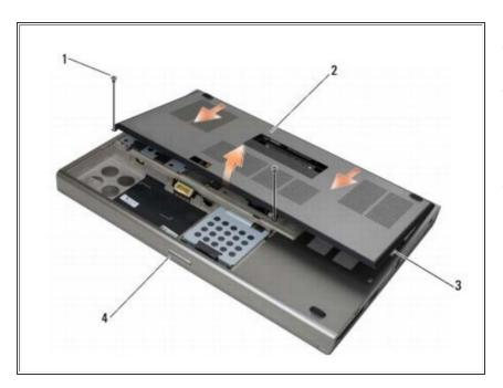
• Remove the two M2 x 3-mm screws.
