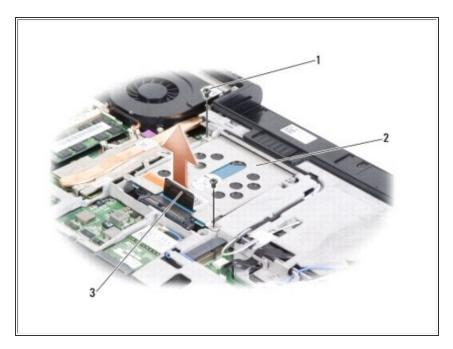
Remove the two screws on the hard drive assembly.
