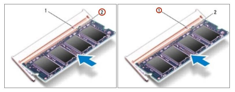
• Align the notch in the memory module with the tab in the memory module connector.
