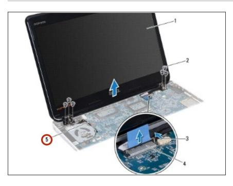
Route the Mini-Card antenna cables through the slot on the computer base.
