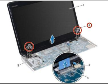
Place the NEW display assembly in position and replace the six screws (three on each side) that secure the display assembly to the computer base.
