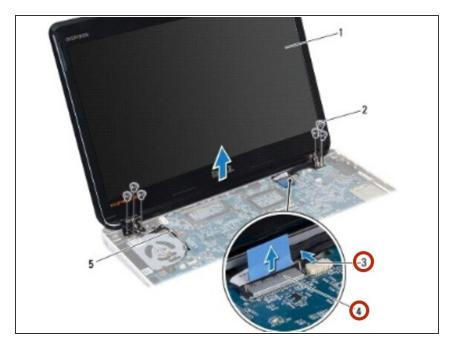
Disconnect the display cable and the camera cable from their connectors on the system board.
