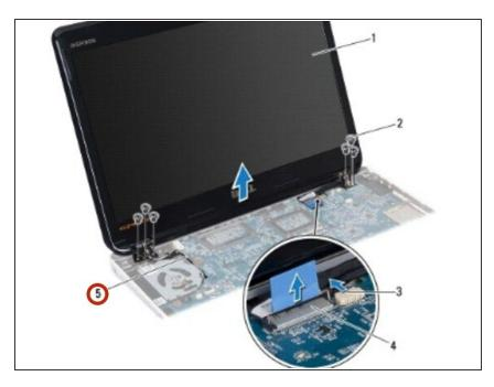
Make a note of the routing of the Mini-Card antenna cables and remove the cables from the routing guides.
