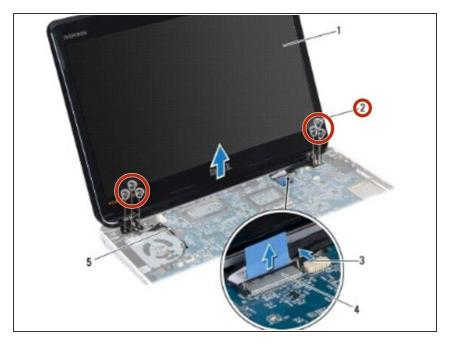
Remove the six screws (three on each side) that secure the display assembly to the computer base.
