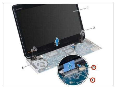
Connect the display cable and the camera cable to their connectors on the system board.
