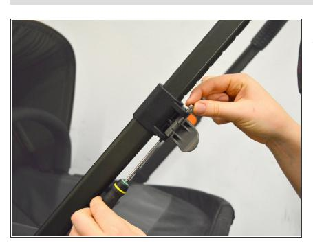
Use the screwdriver to push the screw up and out of the black part.
