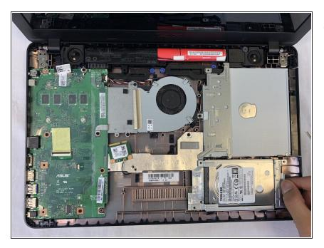
Remove the hard drive by pulling it towards the right, and removing it from the laptop case
