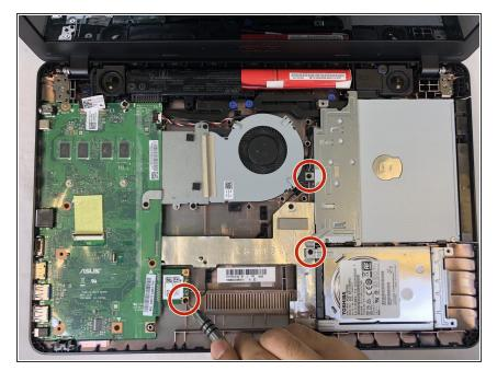
Remove the three 6mm Phillips #0 screws from the motherboard.
