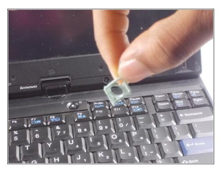
• Grab and pickup the square shaped component. This is the part that you can clean out.
