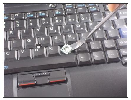
• Again with the pry method, pry up the below component below the key.
