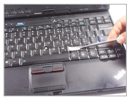
• Use a metal spudger or a flat head screwdriver to pry up the desired key.
