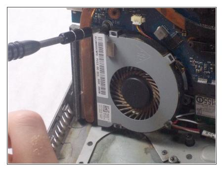
• Located on the lower left, remove the 4mm PH1 Philips screw to the top of the fan.
