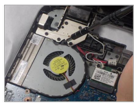
• Remove the 4mm PH1 Philips screw to the top of the fan.
