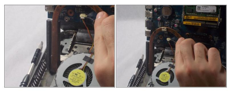
• Remove the wire for the fan by pulling or pushing the white tab from the white box.
