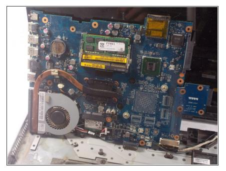
• Remove the motherboard from the USB sockets to the left by first pulling the motherboard to the right and then flip the motherboard up against the screen.
