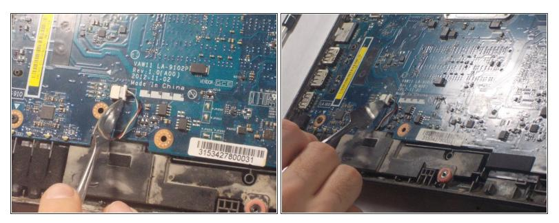
• Located on the lower left of the motherboard, disconnect the wire that connects the speaker by pushing it or pulling it away from the white box.
