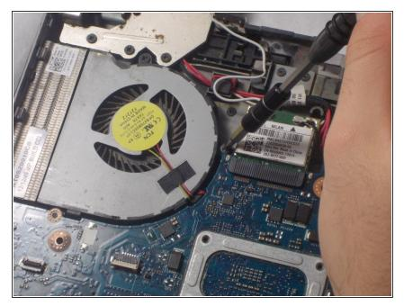
• Remove the 4mm PH1 Philips screw to the right of the fan.
