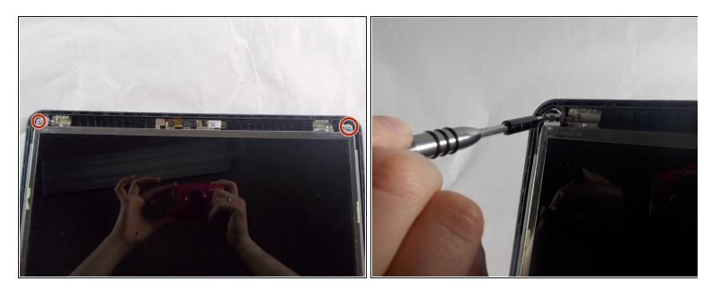
• Unscrew the two 2.5x4 mm screws from the top of the screen.
