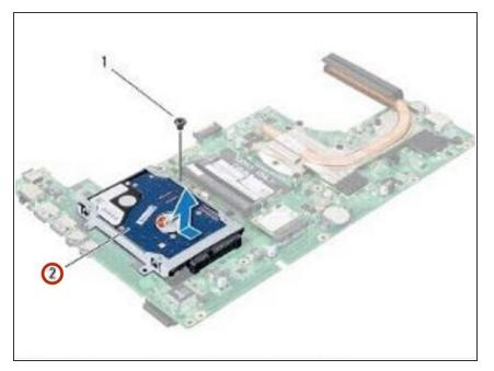
• Place the hard-drive assembly on the system board.
