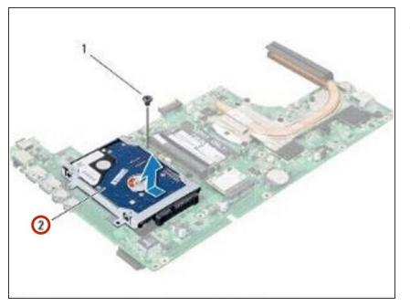
Slide and disconnect the hard-drive assembly from the connector on the system board as indicated in the illustration.
