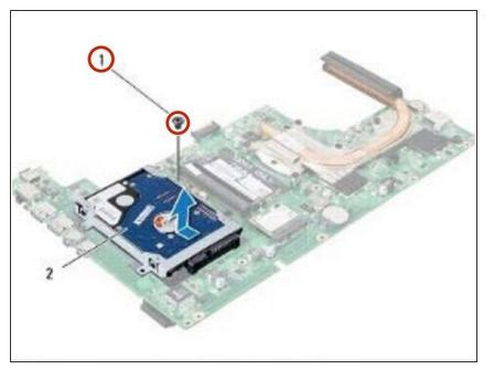
Replace the screw that secures the hard-drive assembly to the system board.
