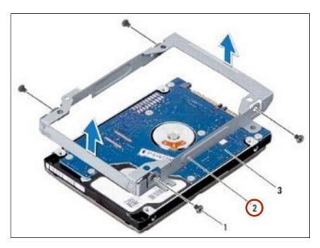
• Lift the hard-drive bracket away from the hard drive.
