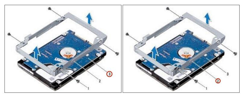
• Place the **NEW** hard drive in the hard-drive bracket.
