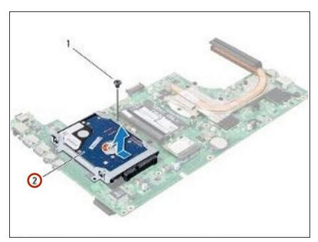
• Slide and connect the hard-drive assembly to the system board connector.
