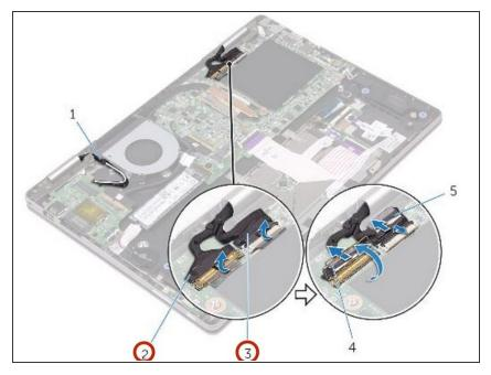
Slide the display cable and the touch-screen board-cable into their respective connectors on the system board and close the latches to secure the cables.
