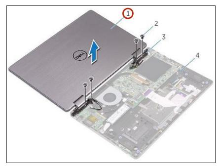
Place the **NEW** display assembly face down on the palm-rest assembly.
