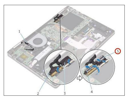
Adhere the pieces of tape that secure the display cable and the touch-screen board-cable to their
