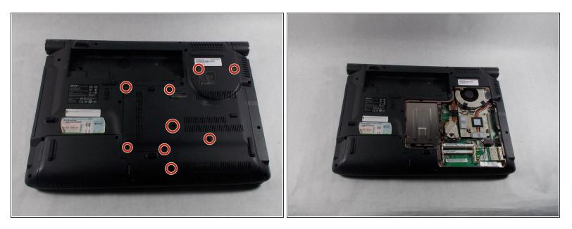
Using a Phillips #1 screwdriver, remove the nine 7mm screws holding the back panel.
