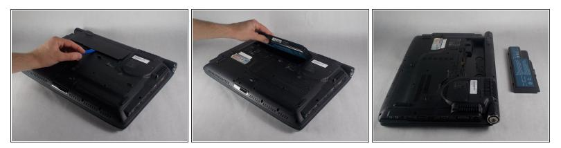
• Pull the battery up and out. Use a plastic opening tool if necessary.
