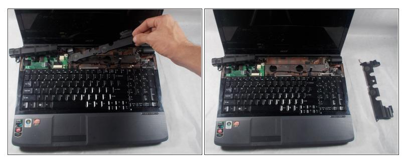
• Lift the speaker from the right side and remove from device.
