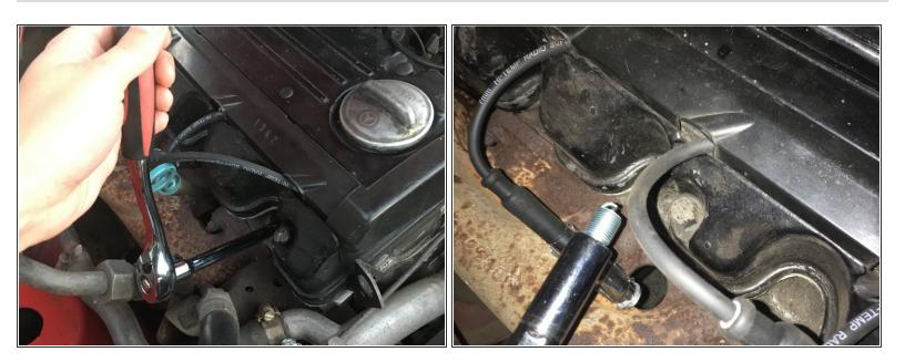
Next, you must use a spark plug wrench. Apply force while twisting counterclockwise, until you remove the spark plug.
