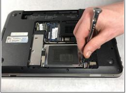
Using a Phillips #0 screw driver, remove the four 4mm screws holding the hard drive in place.
