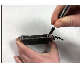
Using a Phillips #0 screw driver, remove the four 4mm screws on each side of the hard drive attaching it to its carriage.
