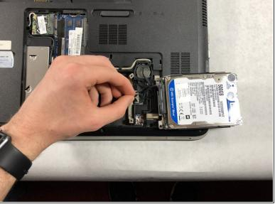
Pull the tab at the end of the cable connecting the hard drive to the laptop.
