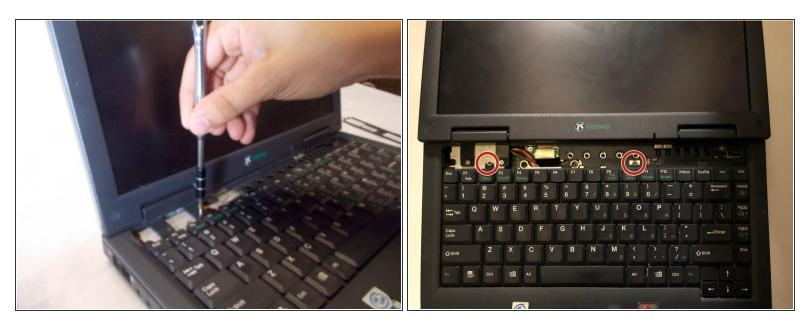
The two J0 screws have now become visible. Using the Phillips J0 screwdriver, remove screws.
