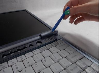
Use a plastic opening tool to lift the back of the hinge cover on the left and right sides of the computer.
