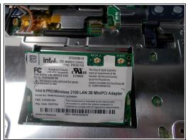
Use tweezers to remove the wires from the Adapter.
