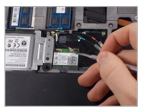
Remove the two wires that are attached to the WiFi card.
