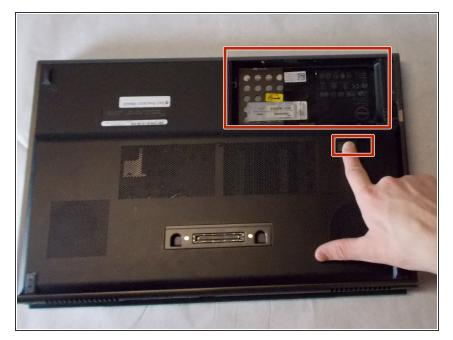
Slide the lock key to unlock the battery. Then you can lift the battery from its holder.
