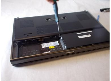
● There are two 1.5mm screws that will be taken off using a Phillips #00 screw driver.
