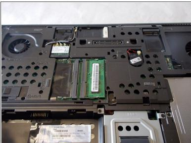
The RAM is held in place by two prongs. By pulling the two prongs lightly away from the chip the RAM is able to be pulled out.
