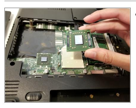
Lift and remove the CPU from the mother board socket.
