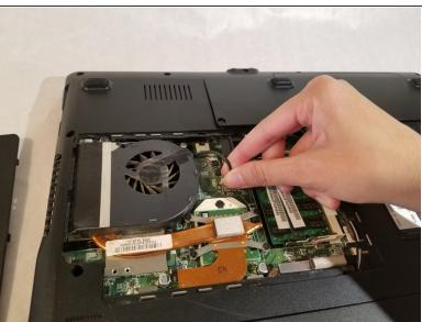
Remove the header by pulling on it with two fingers.
