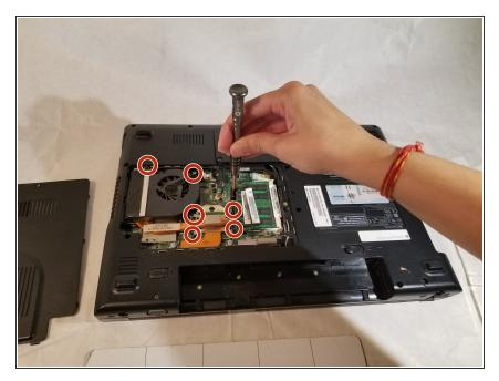
Remove the six 2.5mm screws using a Phillips #1 screwdriver.
