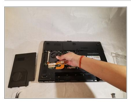
Remove the fan by moving it to the side and lifting it out of the computer.
