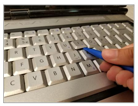
• Using the plastic opening tool, apply force to pry the key upward.
