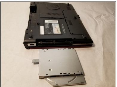
Remove the CD drive from the device.
