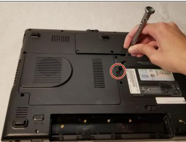
Using the Phillips #1 screwdriver, remove the indicated 6mm screw holding the CD drive.
