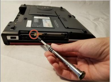
Using the screwdriver, push the release button for the CD drive.
