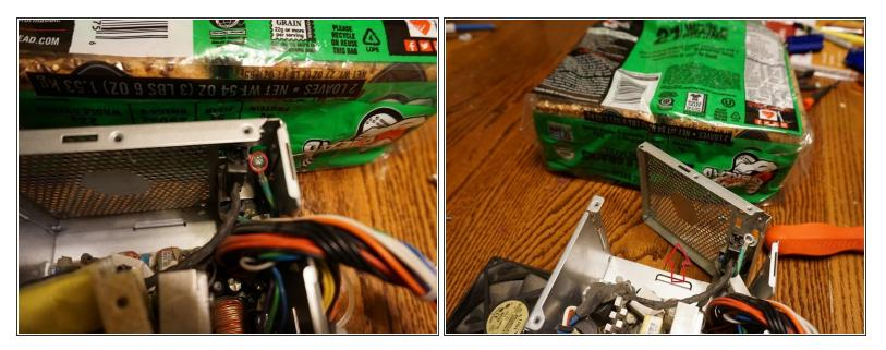
Remove a screw on the back end(with the stair pattern facing towards you) to free the back panel(partially)
