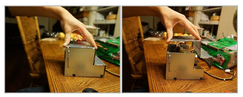
• Here you can now remove the top of the power supply case
