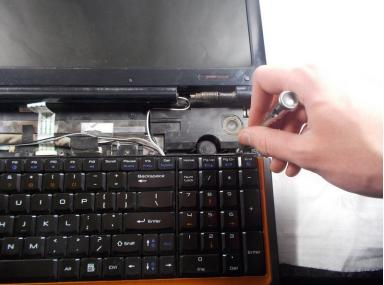
• Remove the five Philips #0 (3mm) screws securing the keyboard in place.
