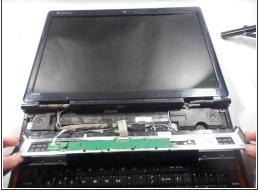
Remove the speaker grill/interaction bar by pulling up at both edges.
