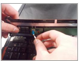
Detach the two ribbon cables on the underside of the keyboard.
