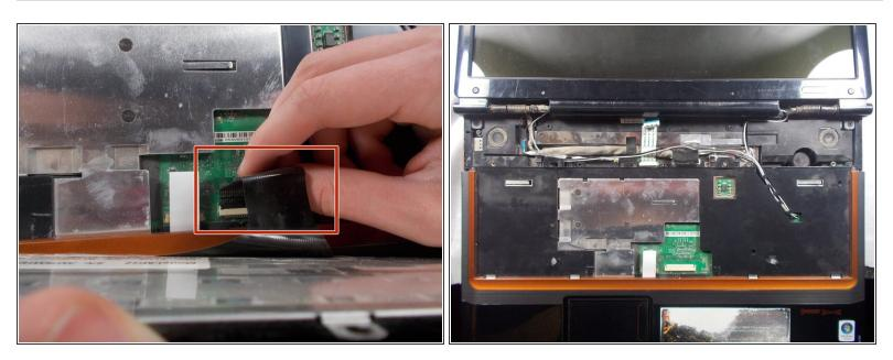
• Remove the ribbon cable attached underneath to the keyboard.
