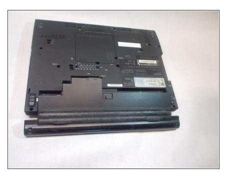
• Then you hold it on unlocked and slide the battery pack out.
