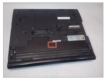
First you push the lock button on the back of the computer from lock to unlock.
