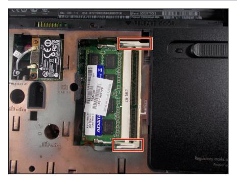
• Unlock the tabs on each side of the ram module. (this lifts the ram module up)
