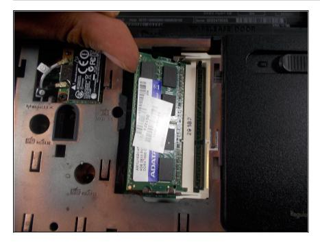
Remove the ram module by pulling it gently away from the slot.
