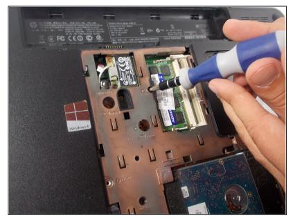
Remove all the screw that secures the keyboard to the computer using a Phillips #0 screwdriver.
