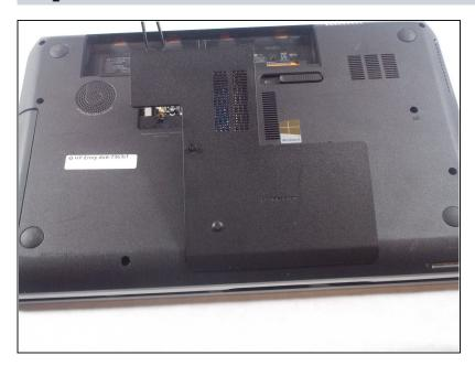
• Lift and remove the back panel of the device.
