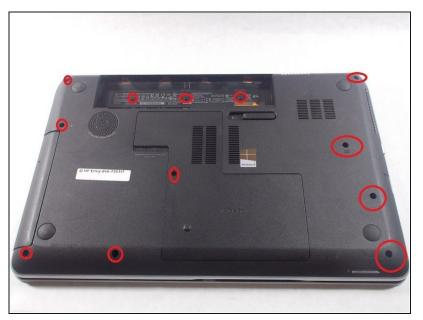
• Remove the circled screws from the back panel.
