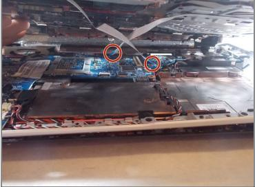
• Flip device right-side-up and remove ribbon cables from plastic cover beneath keyboard. Remove plastic cover from device.
