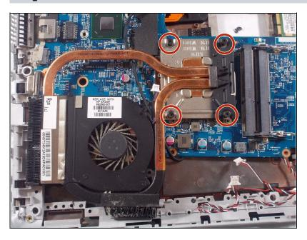
Remove circled screws from blue circuit board and lift fan assembly out of device.
