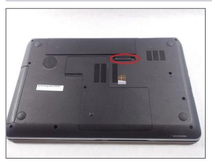
Push the lever underneath the battery to the left.
