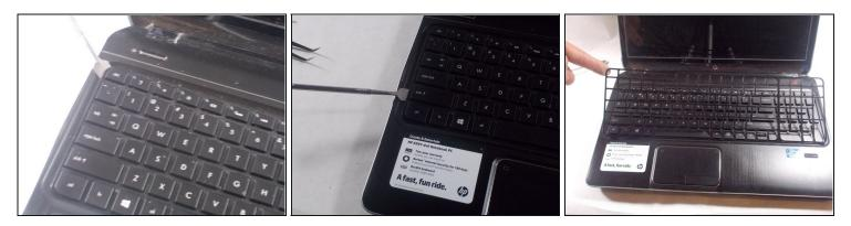
• Flip the laptop back over and carefully pry the keyboard frame out of the device.
