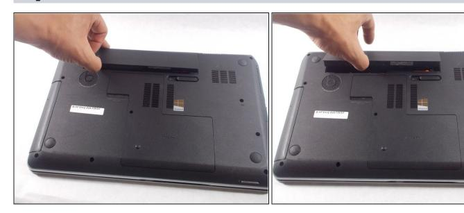
• Lift the battery up out of its socket.
