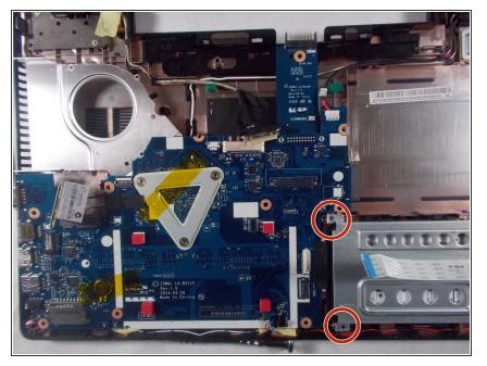
Remove the 2 #1 Phillips screws, then slide the metal cover back and away
