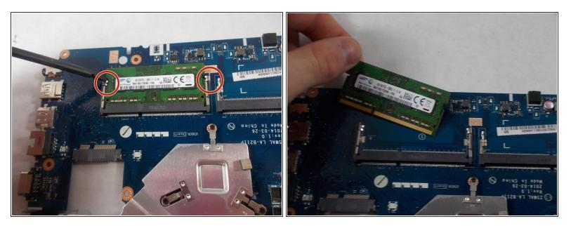
• Press down on the spring clips on either side of the ram, It will unlock and can be removed
