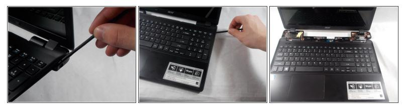
• Flip over the laptop, Using the spudger separate the body of the keyboard from the base of the laptop.
