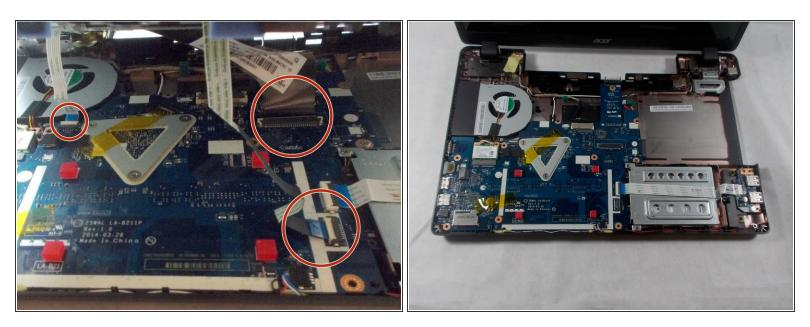
Carefully lift the keyboard and disconnect the 3 ribbon style connectors from the computers boards.
