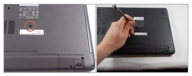
• Remove the 1 screw just above the battery with a Phillips #1 screwdriver.
