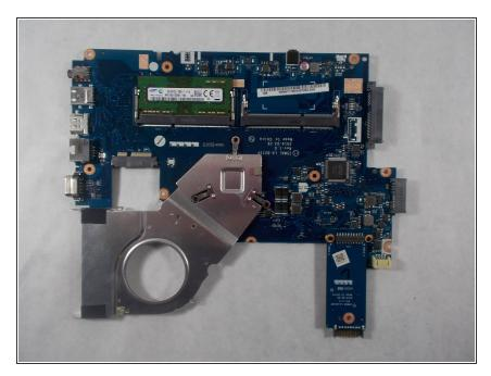
• Remove the board from the laptop body, flip over for access to the ram
