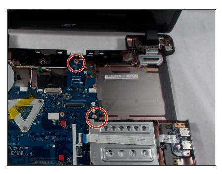
• Remove the last 2 #1 Philips screws from the body
