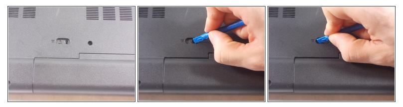
• On the back of the laptop, there is a sliding lock. Push the slider and the battery will unlock
