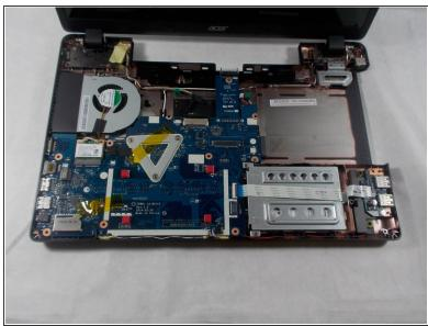
Carefully lift the keyboard and disconnect the 3 ribbon style connectors from the computers boards.
