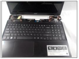
Flip over the laptop, Using the spudger separate the body of the keyboard from the base of the laptop.
