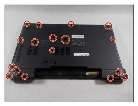
Remove the 17 Phillips #1 screws remaining on the back side of the laptop
