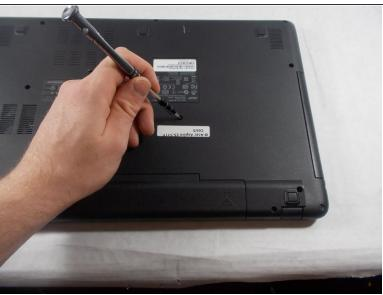
Remove the 1 screw just above the battery with a Phillips #1 screwdriver.
