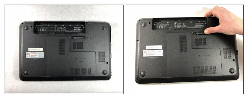
Begin removing the bottom cover by sliding the battery removal slider to the right to pop off the top
