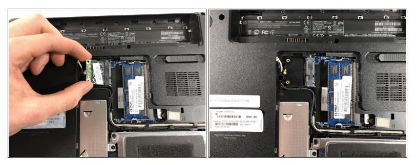
Always handle the WiFi Adapter by the edges to avoid damaging the part.
