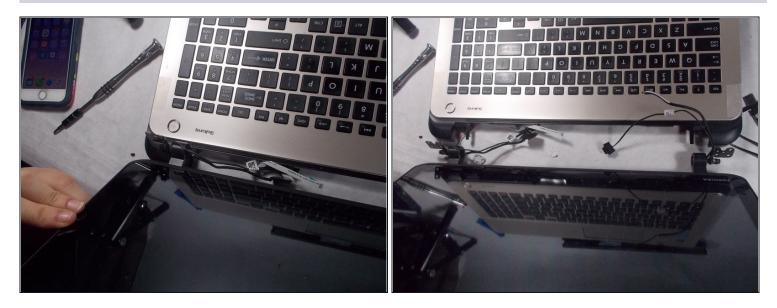
• Gently pull the screen to disconnect the monitor from the hinges.
