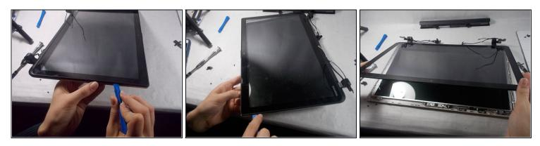
• Use the plastic opening tool to pry the plastic covering off of the monitor.
