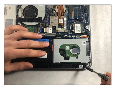
Find and remove the four .4cm phillips head screws holding the hard drive in place.
