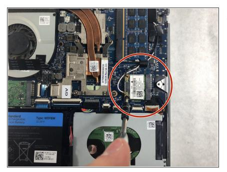
Find the .3cm Phillips head screw holding the WiFi Card in place and remove it.
