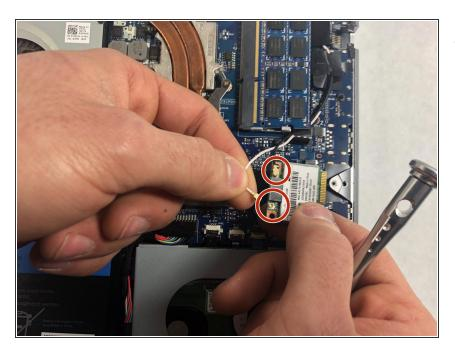
Gently tug on the two wires connected to the Wifi card
