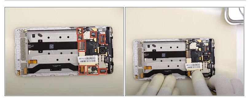
Use a spudger to disconnect all marked ribbon cables.
