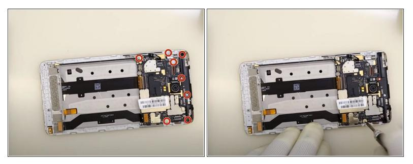
Use a Phillips #00 screwdriver to remove the eight screws fastening the motherboard to the phone's interior.
