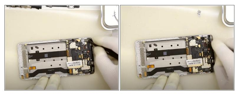
• Use a pair of tweezers to remove the small metal piece from the top of the motherboard.
