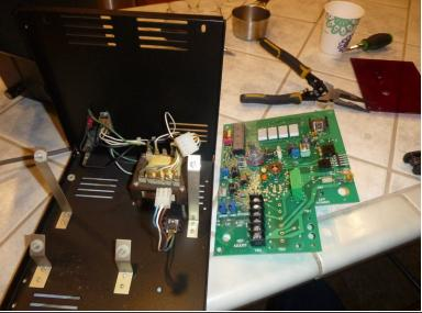
Unscrew all the nuts shown using an adjustable wrench to remove circuit board
