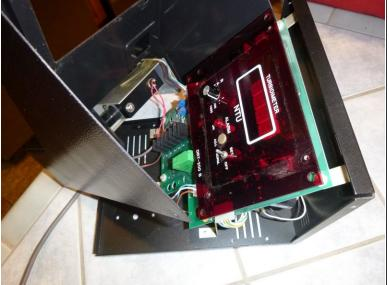
Now unscrew the 4 screws on the face plate and you will be able to lift the cover off the meter but be carful as there are a few plugs and screws left for you to remove
