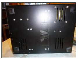
first thing u want to do is take out the two screws on each side of the meter and also take out all the screws on the bottom you will need a philips head screw driver
