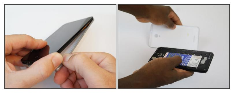
Remove the back cover by sliding your fingernail in the grove around the edge of the phone and prying it off.
