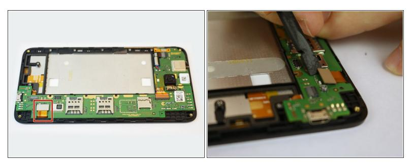
Use the flat end of a spudger to disconnect the ribbon cable.
