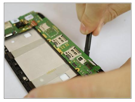
• Use the flat end of the spudger to pry off the motherboard.
