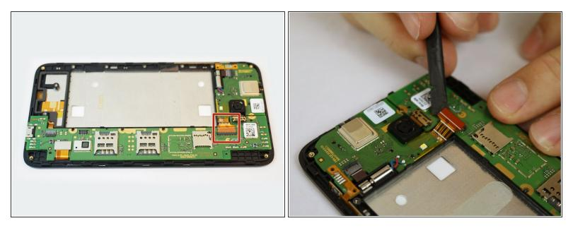
• Using the flat end of the spudger to disconnect the ribbon cable.
