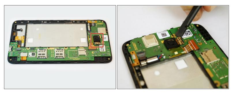
Using the flat end of the spudger, disconnect the camera from the motherboard.
