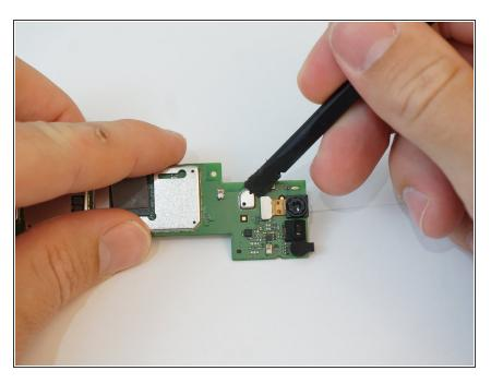
Disconnect the camera from the motherboard using the flattened of a spudger.
