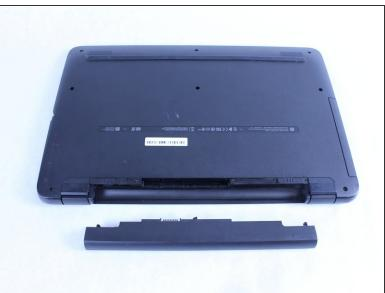
Remove the old battery by pulling it towards you. Replace the old battery with the new one and follow these steps in reverse order to reassemble your device.
