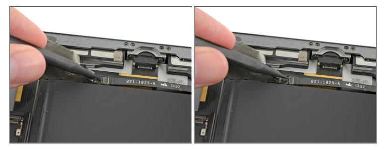
• Use the pointed end of a spudger to flip up the retaining flap on the left speaker cable connector.
