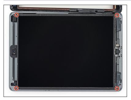
• Remove the four Phillips #00 4.3 mm screws securing the LCD.
