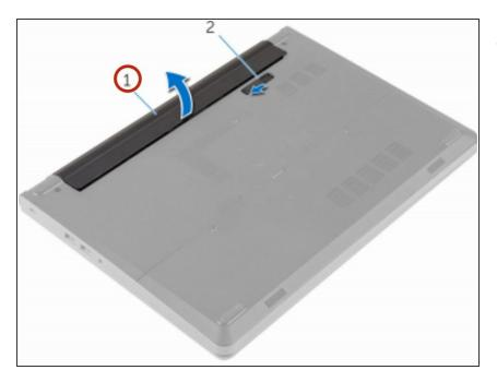
Lift the battery at an angle and remove it from the battery bay.
