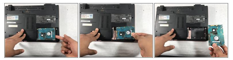
• Detach the hard drive by disconnecting it from the motherboard, pulling it gently from left to right.
