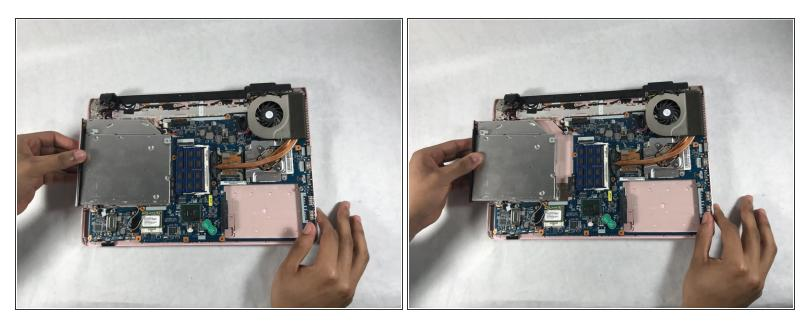
• Slide your finger from the right of the optical disc and pull the optical disc from right to left.
