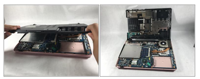
• Lift the backplate from bottom right and left corner and remove it from the laptop.
