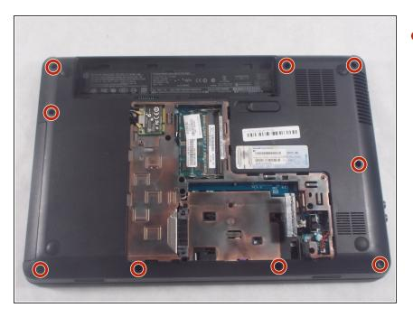
Unscrew all nine 6.0mm JIS #0 screws located on the border of the back panel.
