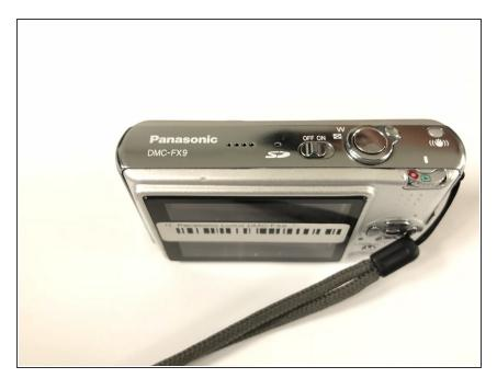
Make sure the power is off by switching the power switch to the left.
