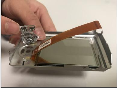
Push on the back panel buttons on the front side to remove the buttons.
