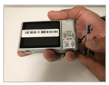
Remove the screws on the right side of the camera by using the Philips #00 screwdriver.
