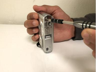
Use a Phillips #00 screwdriver to remove the screws on the left side of the camera.
