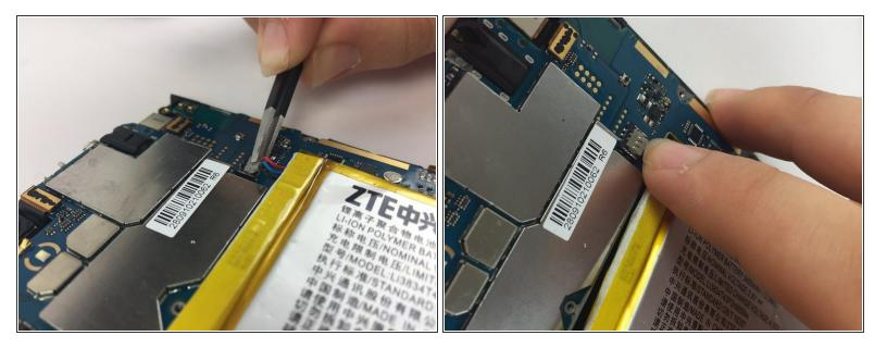
Disconnect the battery from the motherboard.
