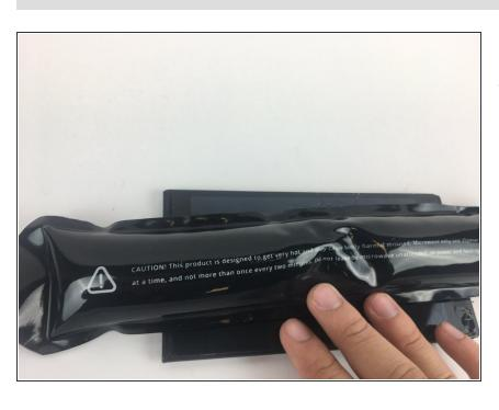
Heat up the iOpener for 30 seconds and place on top of the phone for 2 minutes.
