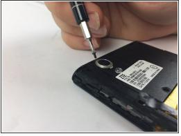
Remove the ten 1.2mm screws with a Phillips #000 screwdriver.
