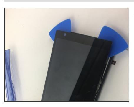
Wedge the opening picks into all the corners of the phone and lift until the screen comes off.
